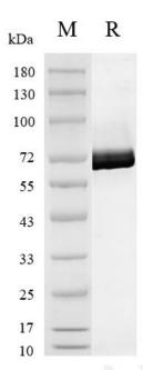
On SDS-PAGE under reducing (R) condition. The gel was stained overnight with Coomassie Blue. The purity of the protein is greater than 95%.
